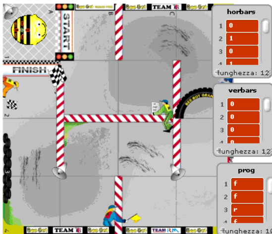
Fig. 4. Simulation in Scratch of a typical scenario with Bee-bot (notice that obstacles and the Bee-bot program are stored in Scratch arrays)
