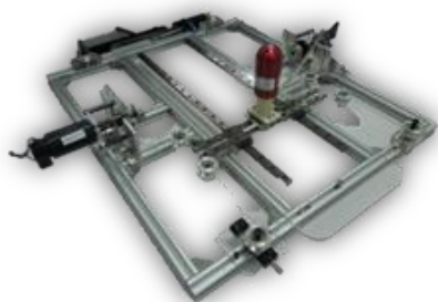
Figure 1: A planar two degrees of freedom end effector robot, H-MAN.
