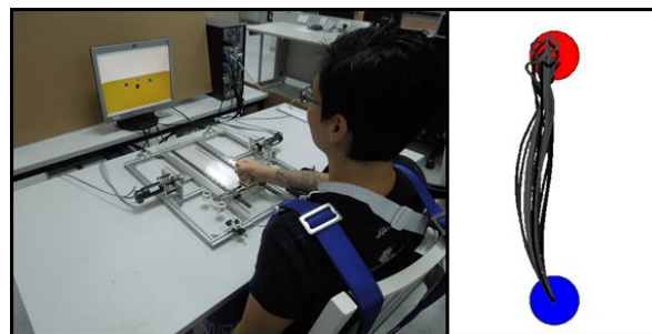
Figure 2: (Left) a participant using H-MAN for training reaching tasks. (Right) Position data collected from HMAN as the subject moves from start to final position.
